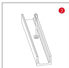
Drive the screw into the aluminum groove
